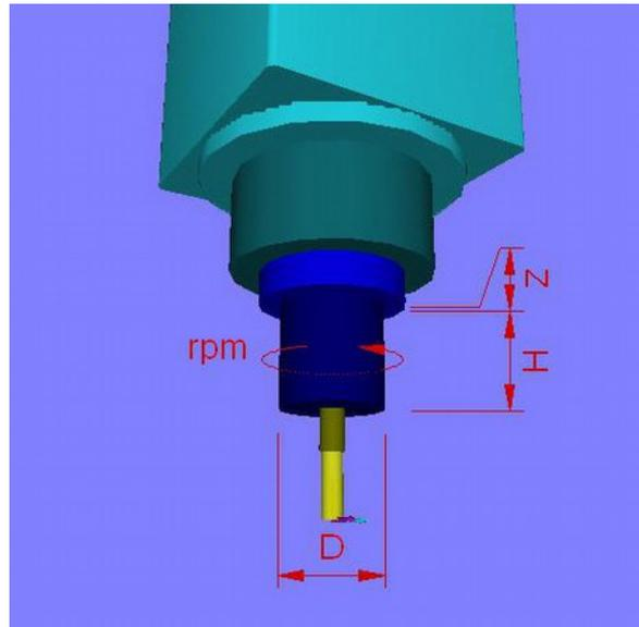
Height  $H$  of the pivot of the spindle. Distance between the spindle tip and the axis of the pivot. This parameter is only active on a machine whose spindle inclines.
