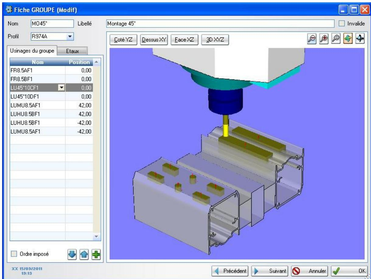
Group name: name of the machining group. Wording: clear description of the machining group. Profile: profile associated with the machining group. Imposed order: forces the machining order (e.g. Roughing then finishing).
