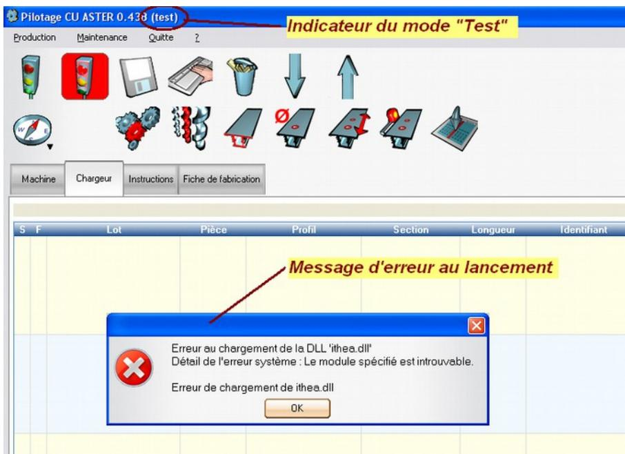
Illustration 4: The driver or the key are not correctly installed
