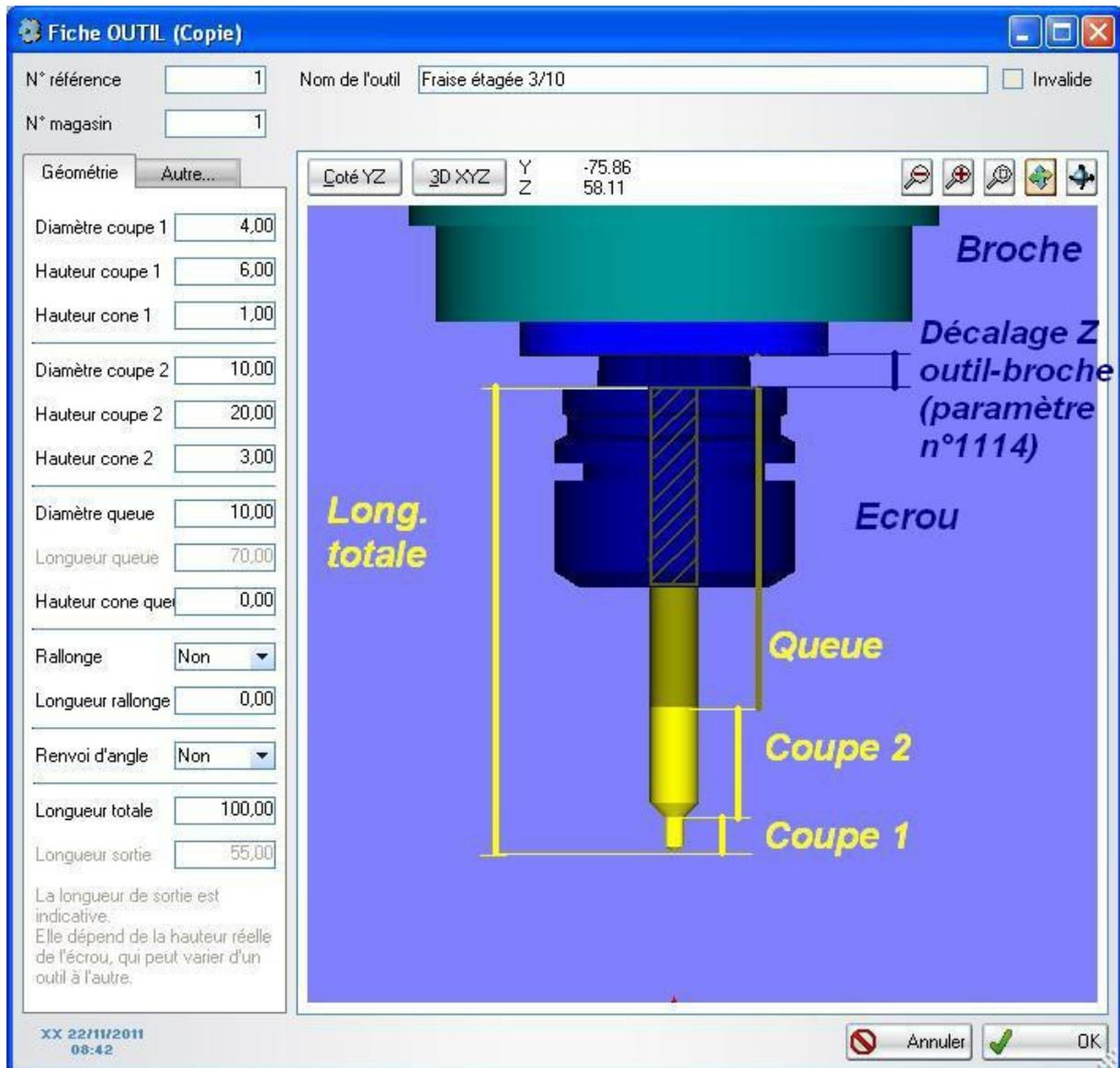
The tool is modelled by 2 cutting zones and a shank. Each zone is composed of a conical part and a cylindrical part. The cylindrical part is defined by a diameter and a length and a tapered part by a height.
