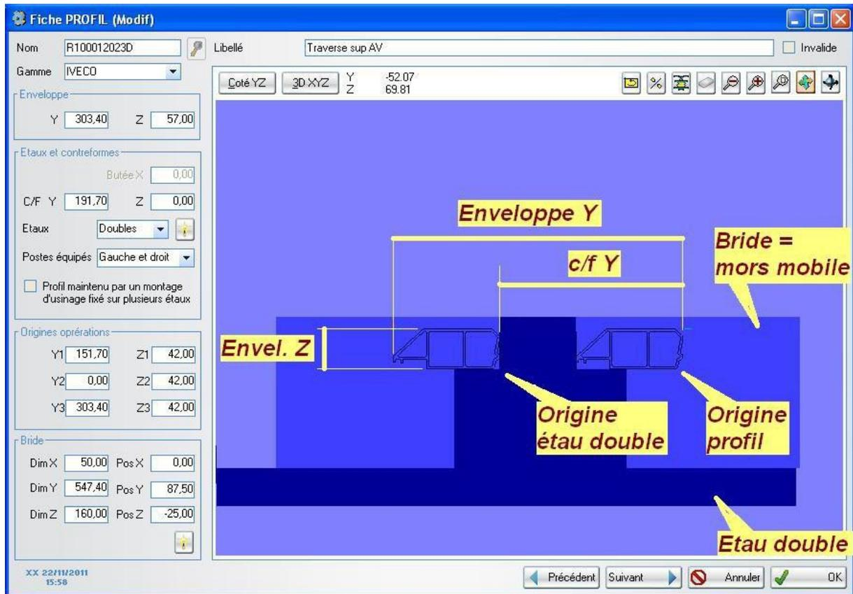
The option “Machining fixture” must be ticked when you place the part in a fixture, itself fixed on the vices. In this case, the vices are positioned by hand by the operator, they are not moved by the shuttle.
