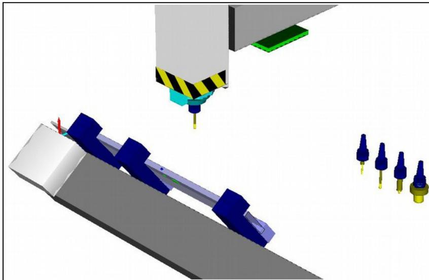
The **PHOENIX** machines are single station units. The spindle is carried by a 3 axis (XYZ) carriage, the part is fixed on a pivoting table around the A axis.
