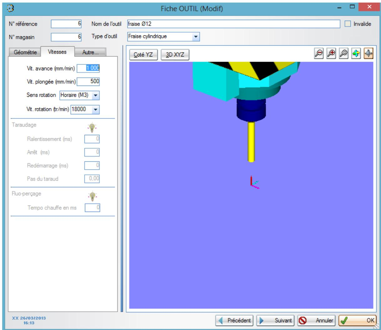
The feed and plunge speed in mm/min are used by the assistants during the creation of the machining operations.
