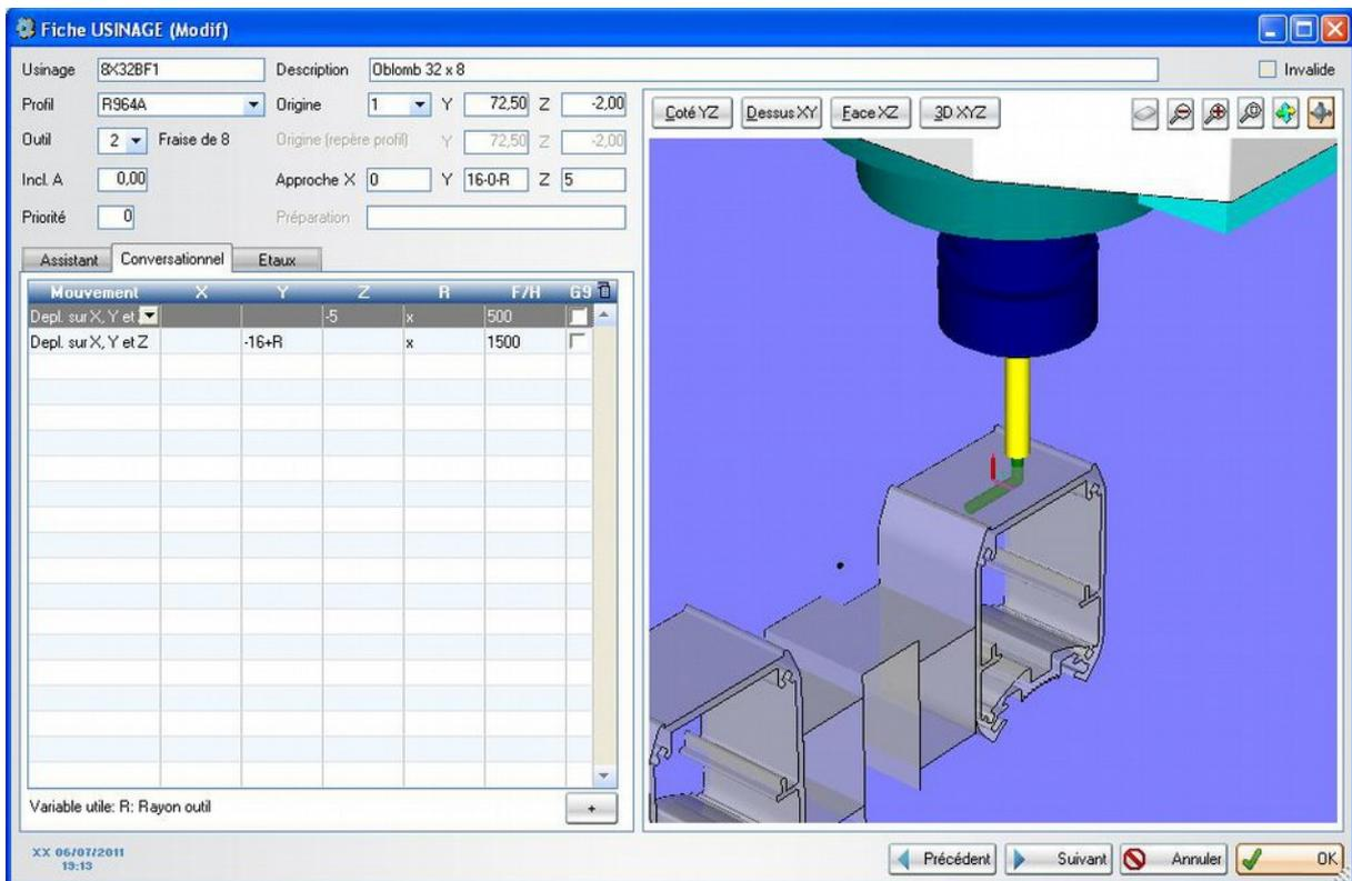
The trajectory is composed of a succession of linear (G1 in ISO), circular (G2 or G3 in ISO) movements and time-outs (G4 in ISO).
