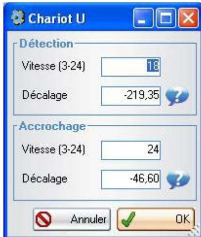
The “detection” frame allows you to set the cycle for measuring the positions of the vices. The higher the speed, the less accurate the detection. The mechanical system for setting the vices in place authorises an error of several millimetres (radius of the centring taper on the positioning pin).
