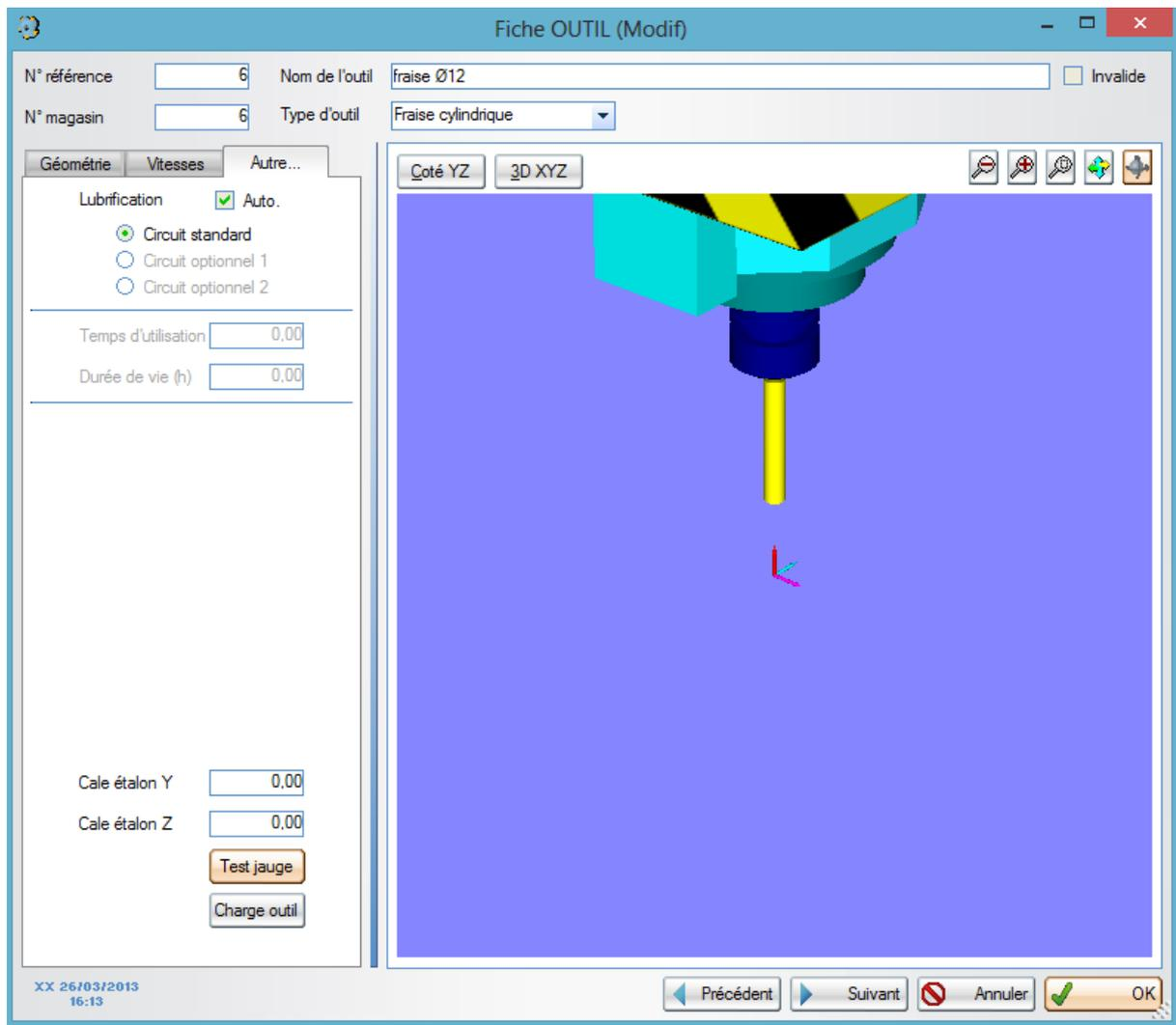
The lubrication can be started systematically during the whole machining cycle or only upon request from the operator.
