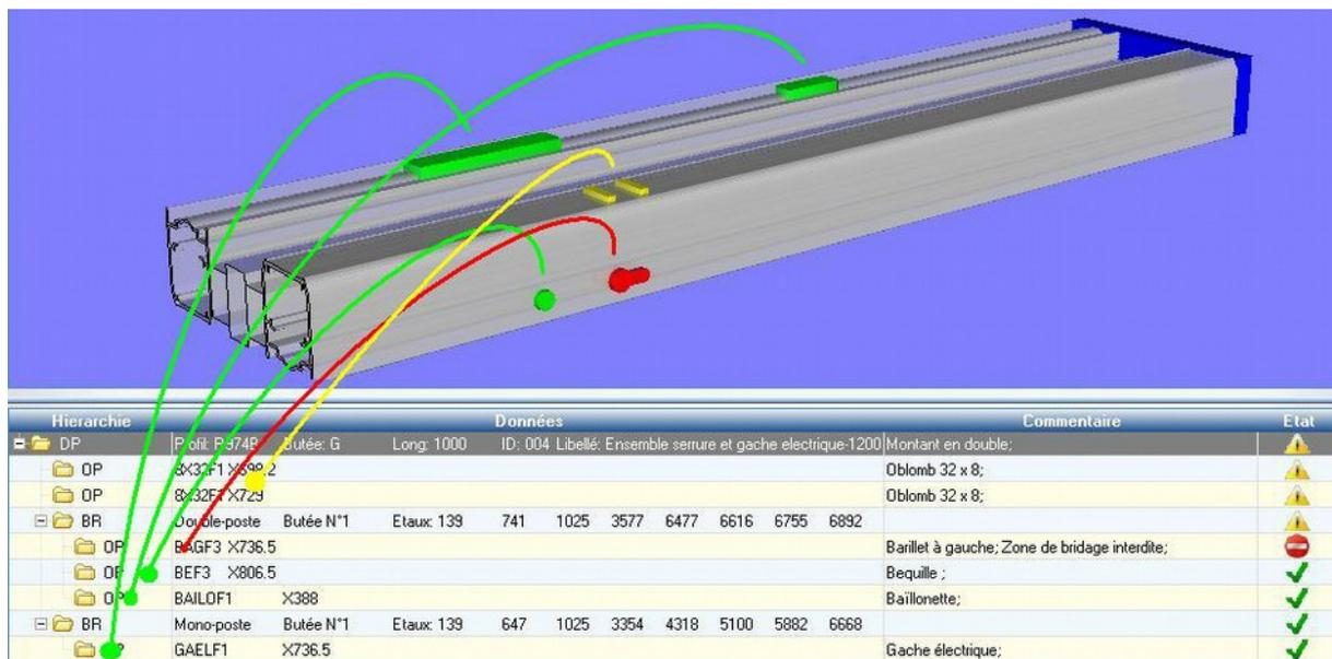
The part is produced in a profile R974B of 1m in stop on the left. The view was turned to display the operations performed on the rear face;
