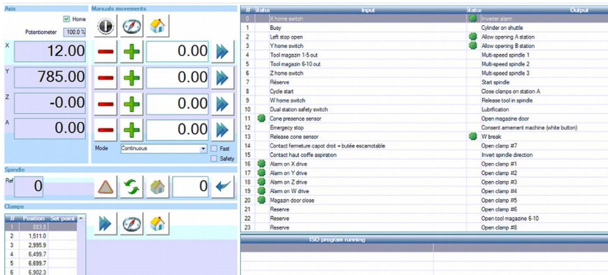
The “Axis” frame provides the status of the POM indicator (a tick indicates that the origin has been set), of the feed potentiometer and the current position of the 4 axes of the machine.
