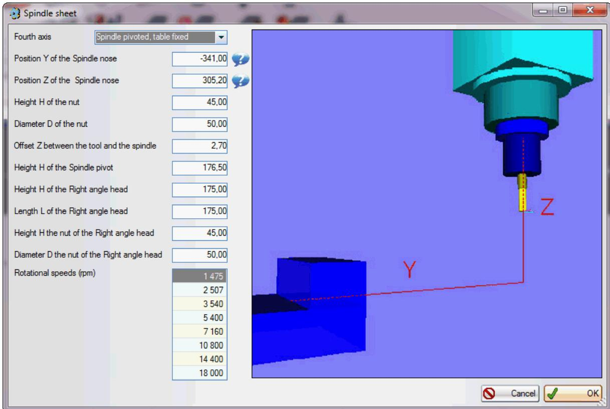
4th axis: To machine on the side of a profile, you can switch over the spindle (case of the Orion unit = spindle on pivot, table fixed) or the part (case of Phoenix unit = spindle fixed, table on pivot)
