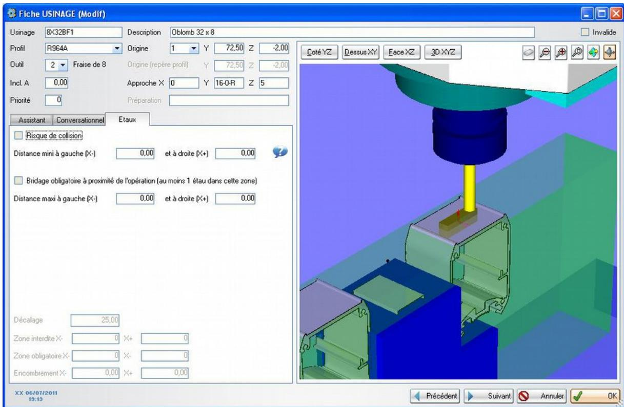
Risk of collision: this option must be ticked if there is a risk of collision between the spindle and the vices. In this case, you must specify the zone forbidden to the vices.
