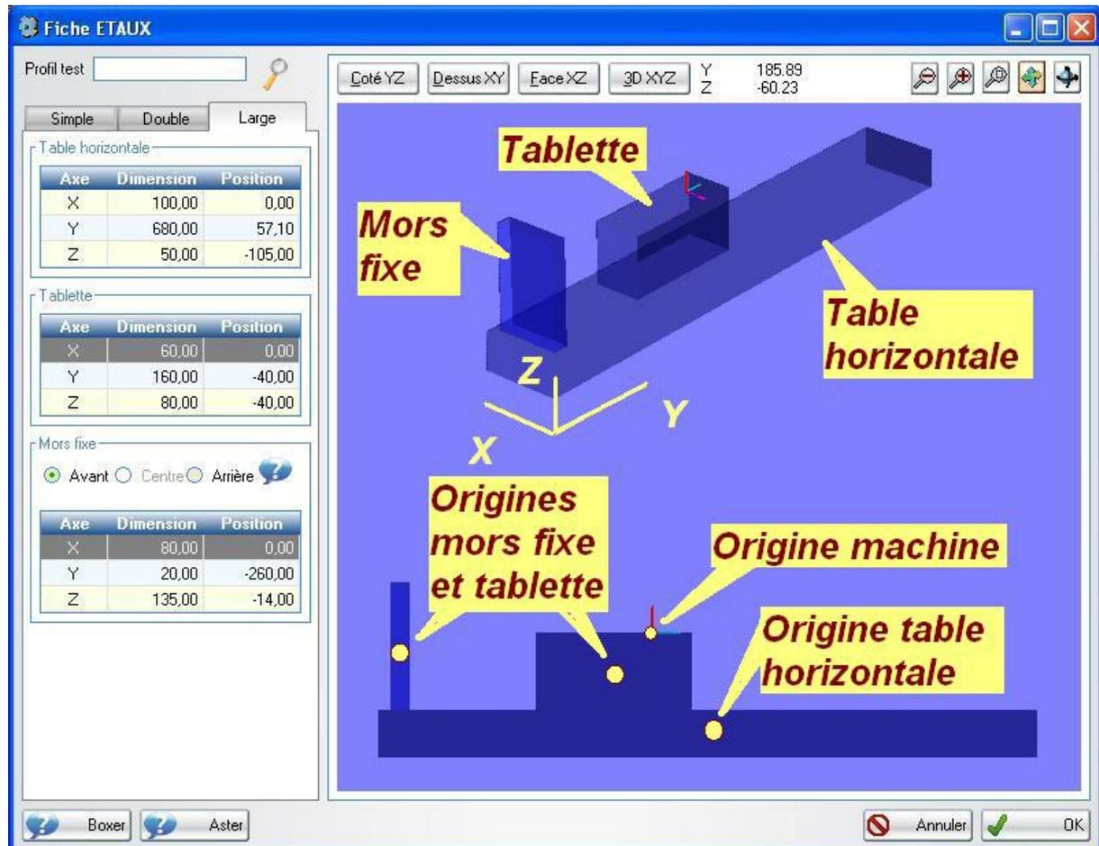
Each model of vice is composed of a horizontal table, a plate and a fixed bit. The horizontal table is common to the 3 variants. Each element is modelled by a parallelepiped for which you define the dimensions and the position of the centre.
